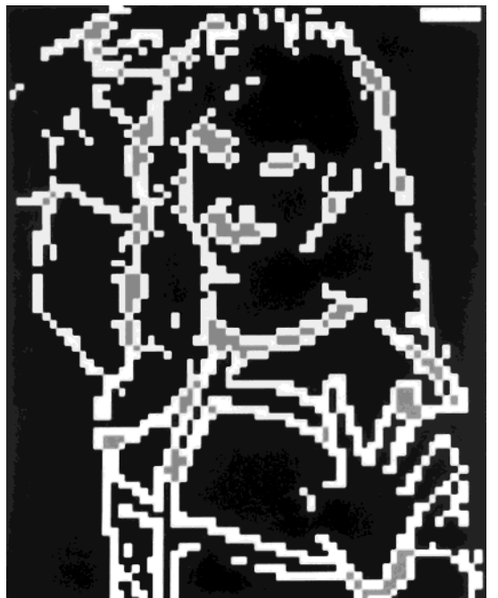
FIG. 5. An example of classification. Light gray, dark gray, and black represent edge, texture, and flat block, respectively.
