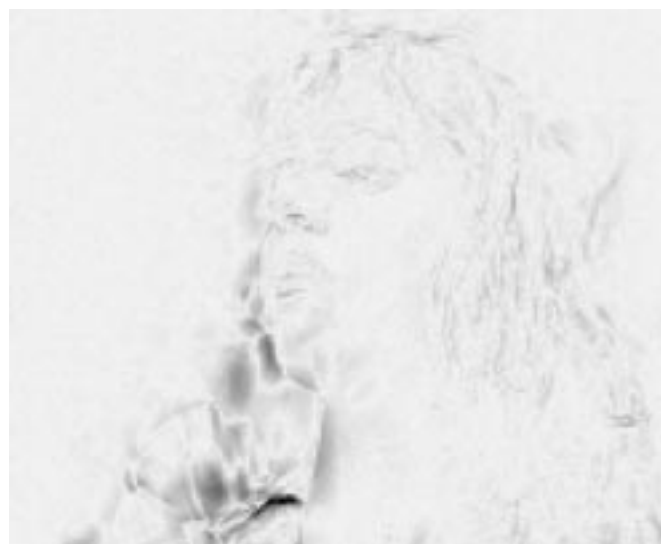
Fig. 8. Fifty-second DFD of the proposed noniterative exhaustive GOBMC-R1 for the Suzie sequence with the bilinear window and PSNR = 32.79 dB.
