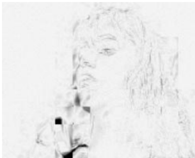
Fig. 6. Fifty-second DFD of block motion compensation (BMC) for the Suzie sequence with PSNR = 30.33 dB.
