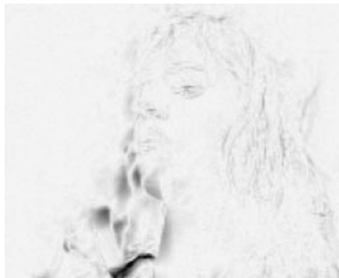
Fig. 7. Fifty-second DFD of BMC vectors with OBMC reconstruction for the Suzie sequence with the bilinear window and PSNR = 31.51 dB.
