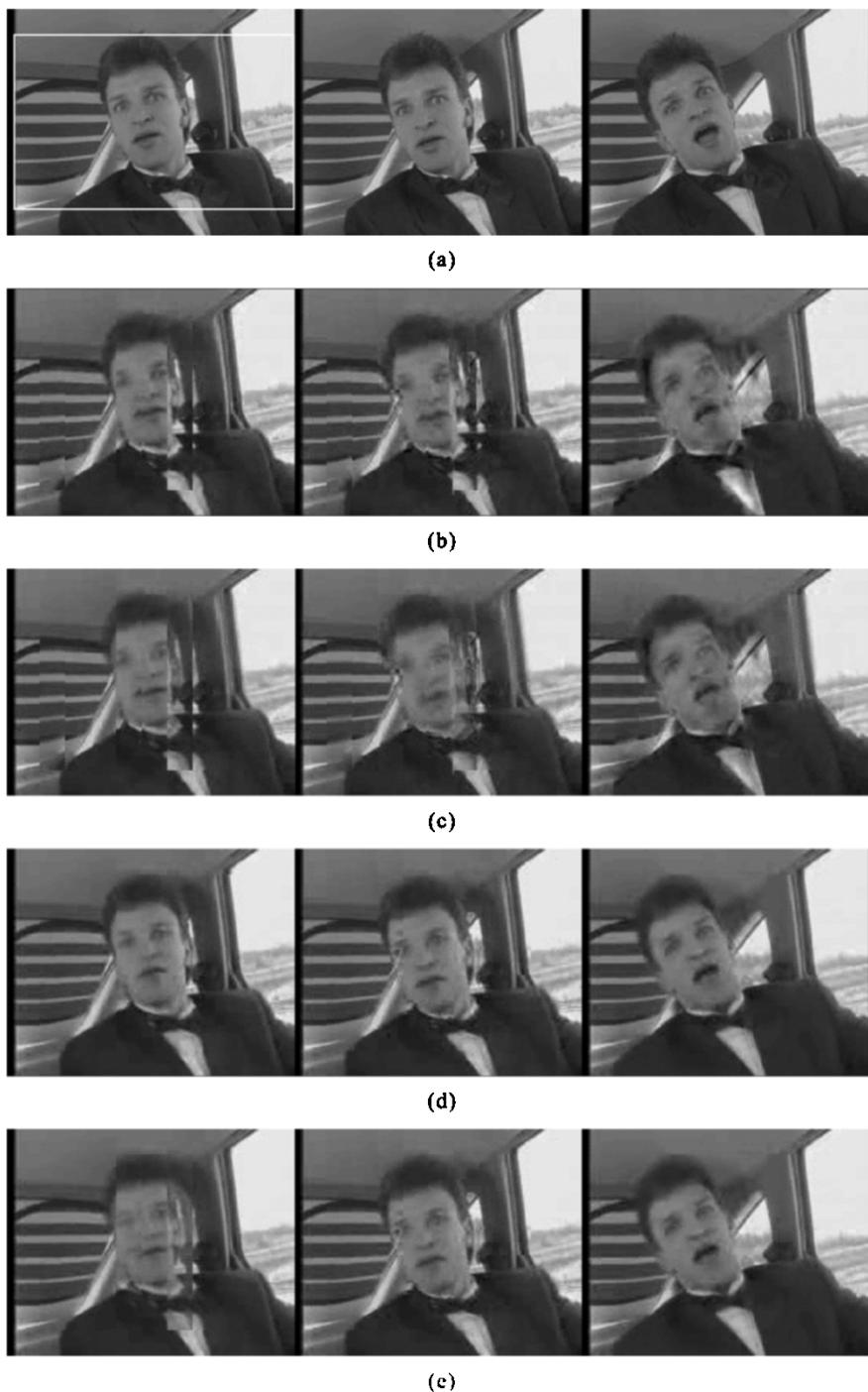
Fig. 3. 10th, 11th, and 35th frames of “Carphone” sequences. (a) Original sequence. Image decoded by using (b) conventional H.263, (c) MMSE H.263, (d) conventional DMC, and (e) MMSE DMC.
