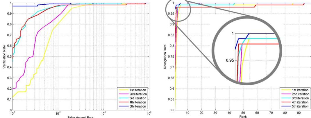
Figure 6. Performance of the 150-to-1 meter face matching result with different enhancement methods: ROC (left) and CMC (right).
