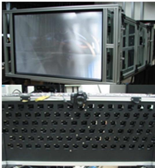
Fig. 11. The 55-in, 100-Mpixel multi-projection 3D display system.
